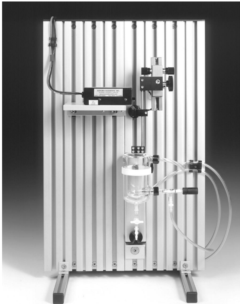
Figure 4 Tissue Bath in Down Position. Lower Tissue Clamp is Fully Exposed.
