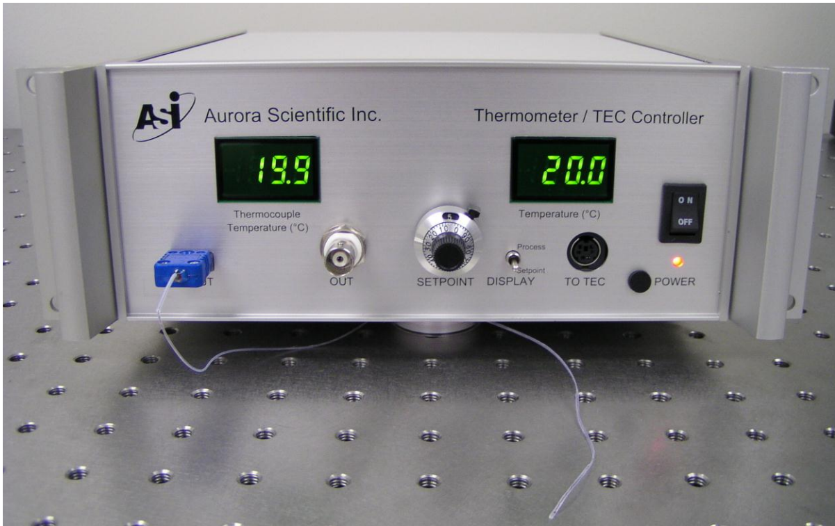
Figure 2 825A TEC Controller
