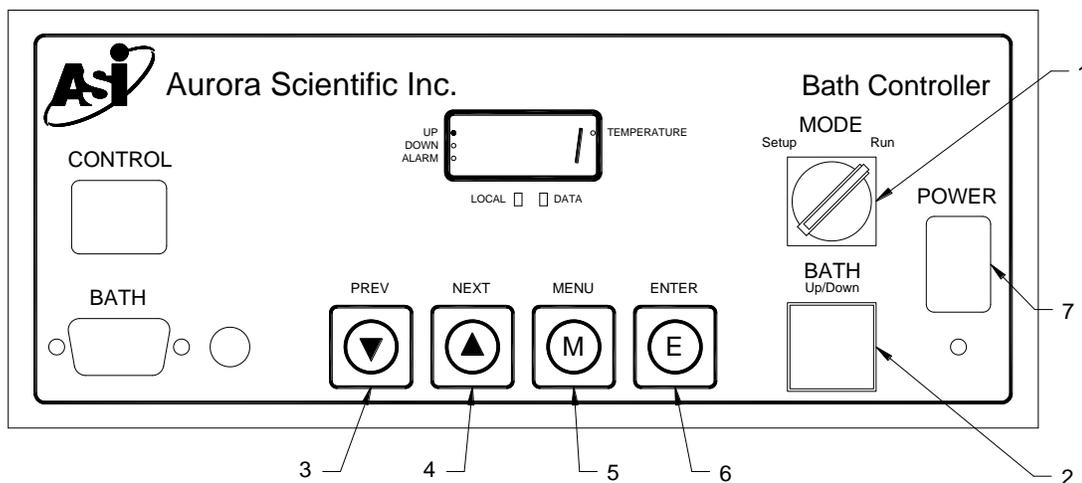
**Figure 4 Diagram of Bath Controller Front Panel**
