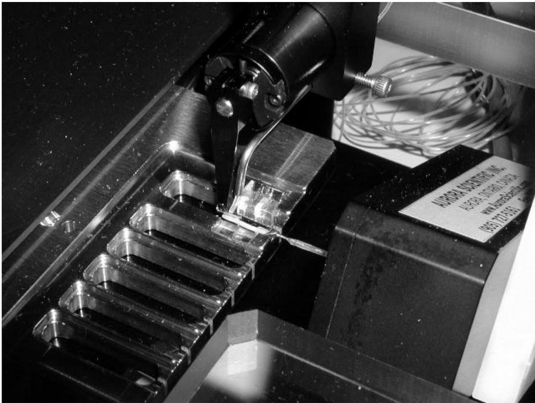
**Figure 3 Close-up of Lever and Force Transducer in Bath 1**
