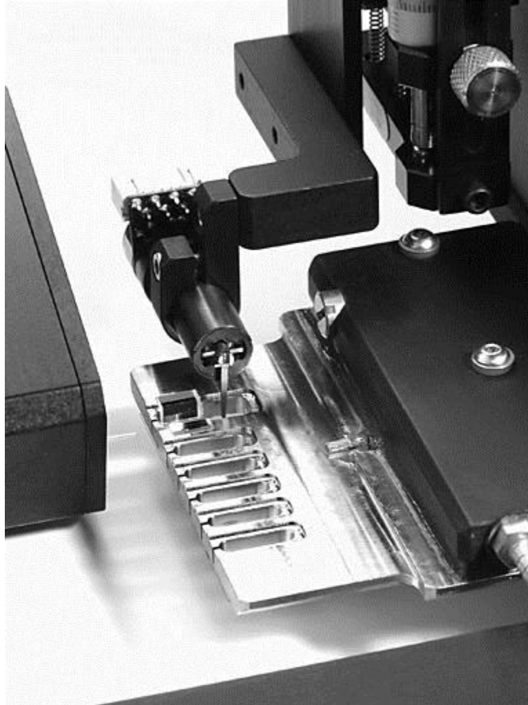
Figure 3 Close-up of Length Controller and Force Transducer in Bath 1
