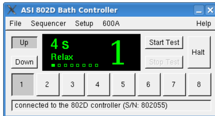
Figure 7 Main Window of 802D Bath Controller Software
