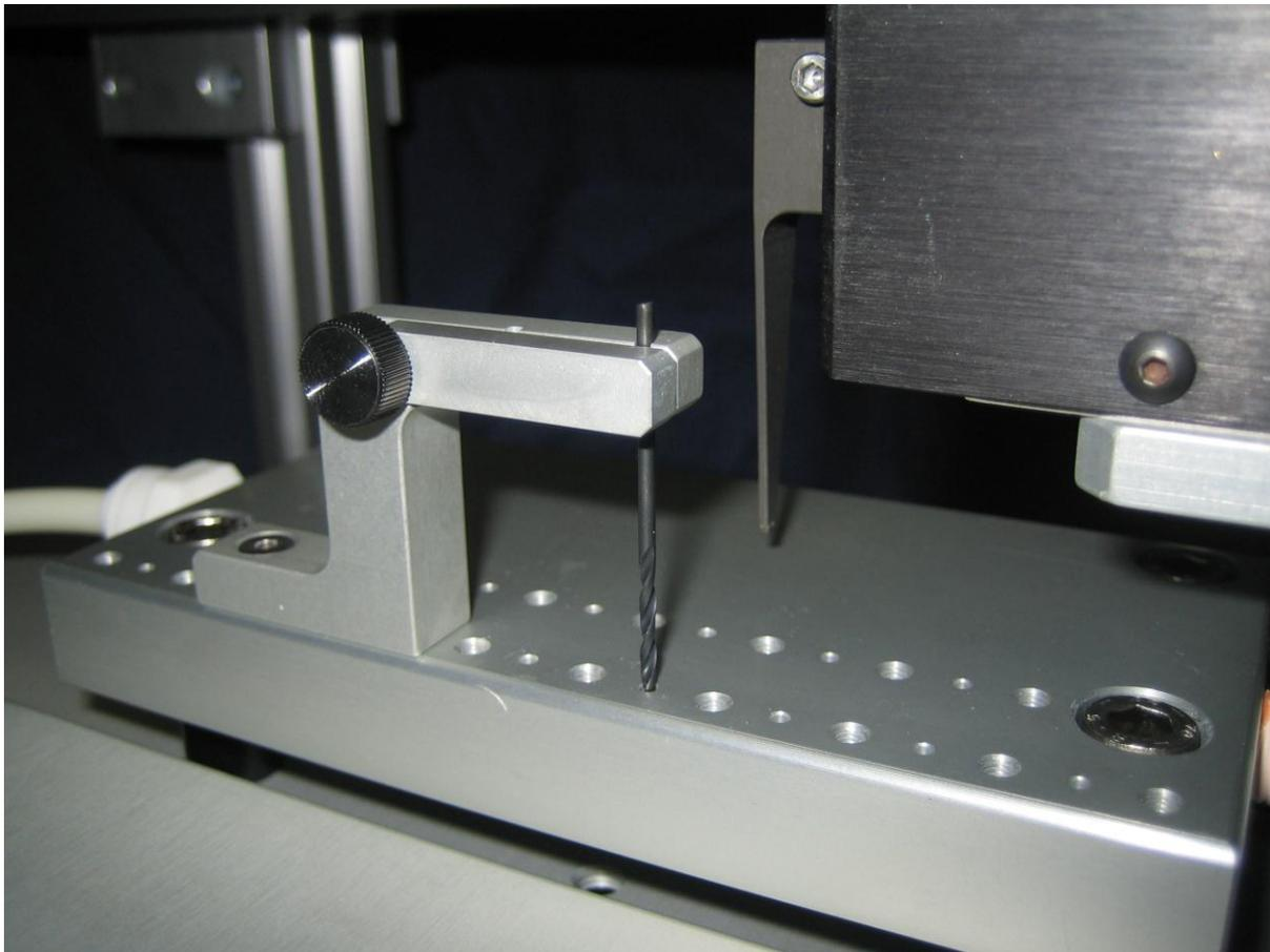
**Photo 3 Limb Plate with Vertical Drill Clamp**
