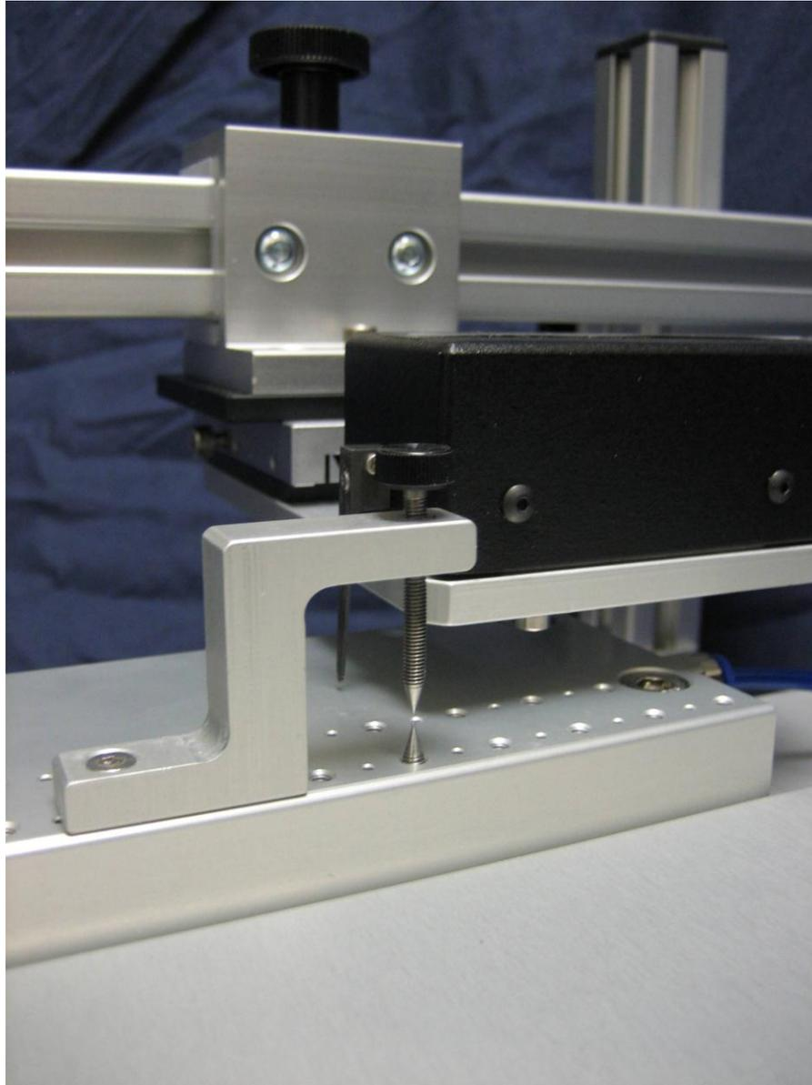
**Photo 2 Limb Plate with Screw Clamp**
