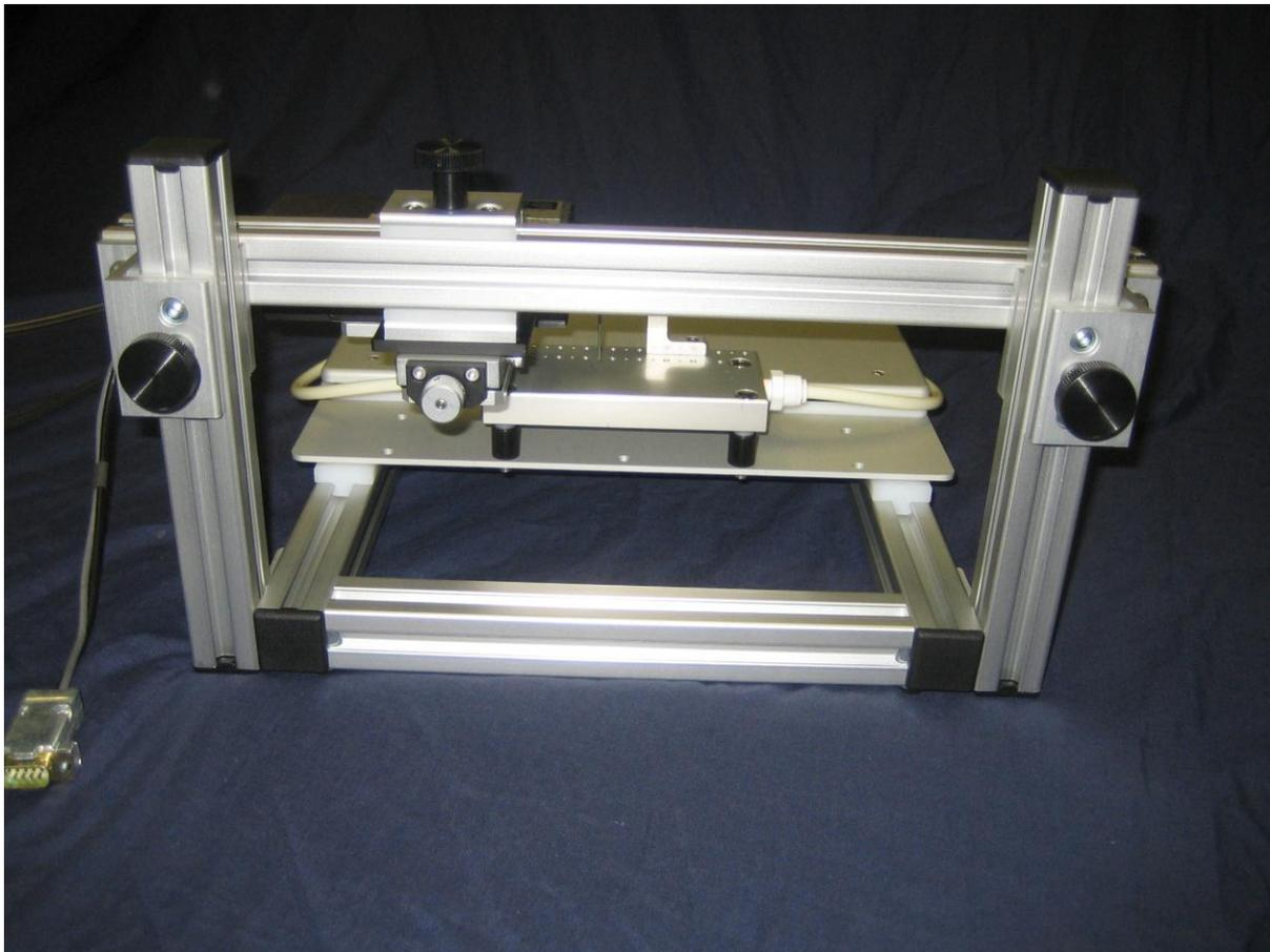
**Photo 4 Back View of 807A Showing Vertical and Horizontal Motor Position Adjustments**
