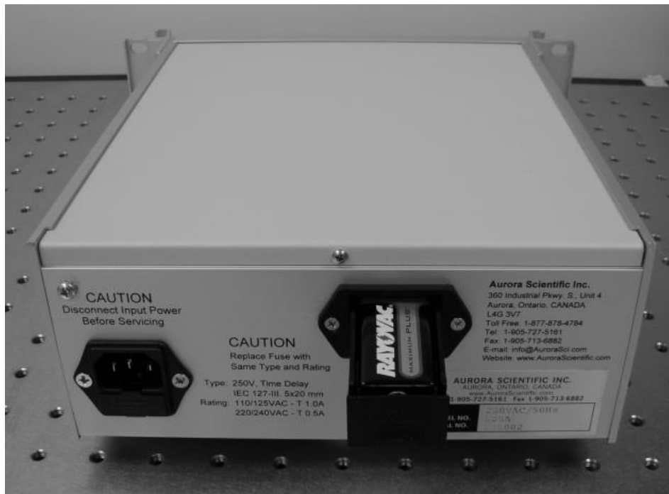
Figure 2: 825A Back Panel with Battery Drawer Open
