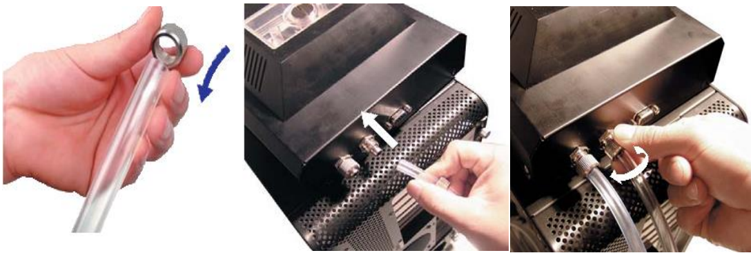
Figure 1: Attaching Hoses to Circulator
