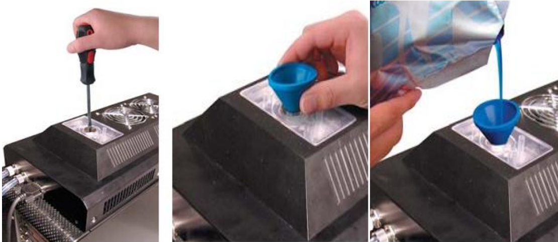
Figure 2: Filling Coolant Reservoir
