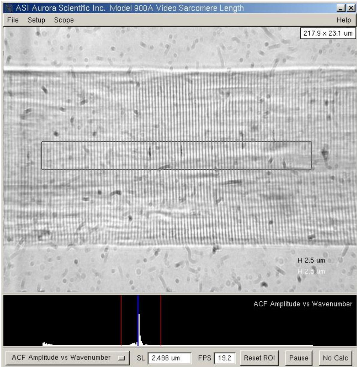
**Figure 4 VSL Main Screen showing the Video Image and the ACF Amplitude vs Wavenumber Graph**
