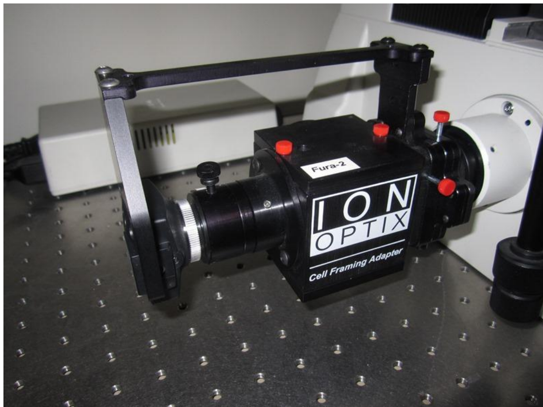
Figure 3 Camera attached to Cell Framing Adapter
