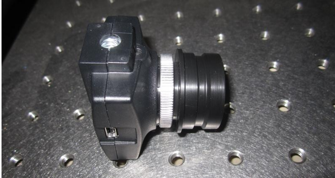
Figure 2 C-Mount attached to camera
