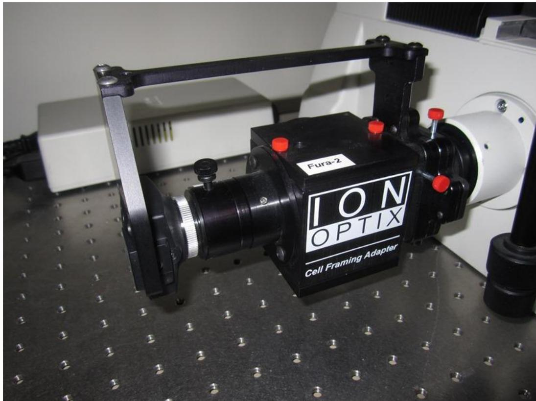
**Figure 3 Camera attached to Cell Framing Adapter**
